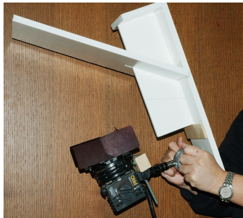
Figure 4: Light source with attached foam-core diffuse reflector used for hand-held data gathering.
