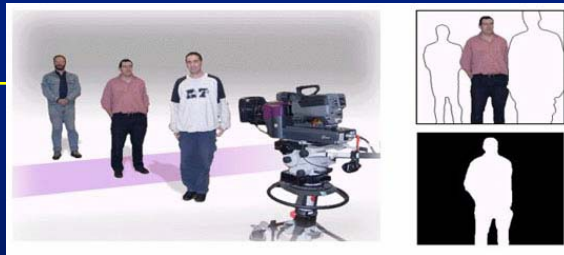
Objects that lay outside the designated range (both near the camera or further away in the background) are not included in the key.
