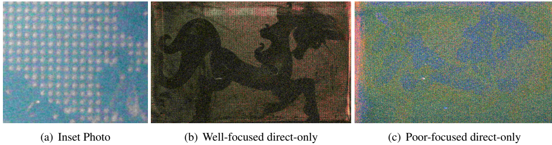
Figure 4-1: Direct-only images by Nayar et al. method for a horse-shaped object enclosed in an aquarium with diluted milk(Concentration 0.11%) (a) Inset of a captured photo with a projected high-frequency pattern (b) Direct-only image in a well-focused case (c) Direct-only image in a poor-focused case
