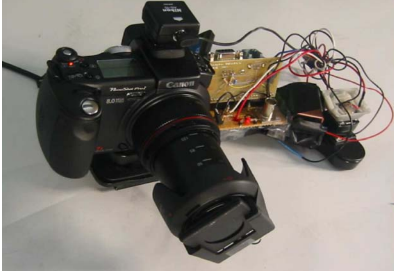
Fig. 9. The flutter shutter camera. The Coded exposure is achieved by fluttering the shutter open and closed. Instead of a mechanical movement of the shutter, we used a ferro-electric LCD in front of the lens. It is driven opaque and transparent according to the desired binary sequence.
