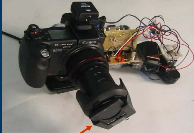
LCD opacity switched in coded sequence
