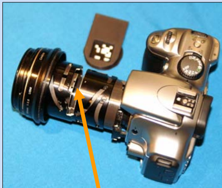
The aperture of a 100 mm lens is modified
