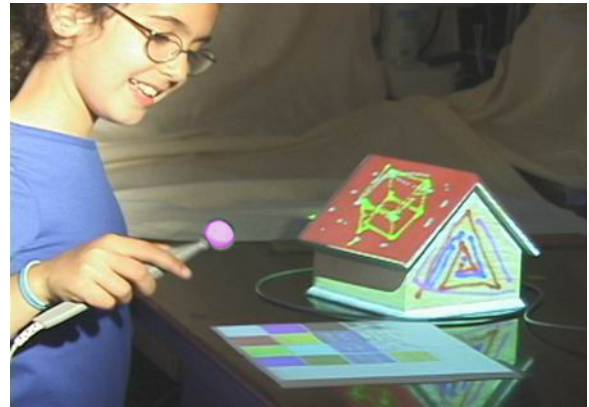
Figure 1: An enthusiastic young user (Miriam Mintzer Fuchs, age 9 years) demonstrates our easy to use system for 3D painting on movable physical objects. Note that the color palette on the table and the color on the spherical tip of the “paint brush” are projected.
