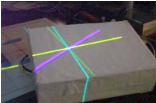
Figure 4: Projector calibration. The two sets of cross hairs give 2D projector coordinates. The corresponding 3D point is measured with a stylus (tracker).
