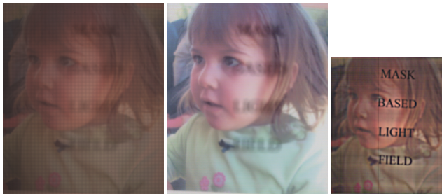
Figure 9: Our heterodyne light field camera can be used to refocus on complex scene elements such as the semi-transparent glass sheet in front of the picture of the girl. (Left) Raw sensor image. (Middle) Full resolution image of the focused parts of the scene can be obtained as described in Section 3.6. (Right) Low resolution refocused image obtained from the light field. Note that the text on the glass sheet is clear and sharp in the refocused image.
