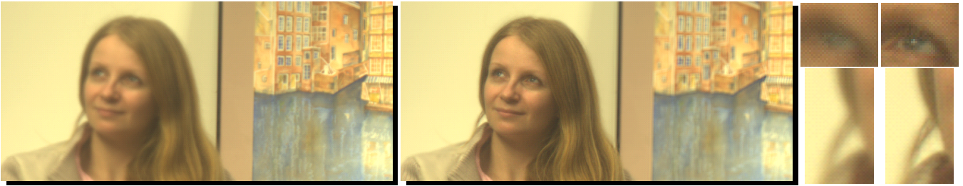
Figure 12: Full resolution digital refocusing using encoded blur camera. (Left) Captured photo where both the person in front and the painting are blurred. (Middle) Refocused image, the person has been brought into focus. (Right) Since the defocus PSF is made broadband by inserting a broadband mask in the aperture, deconvolution can recover fine features such as the glint in the eye and the hair strands.
