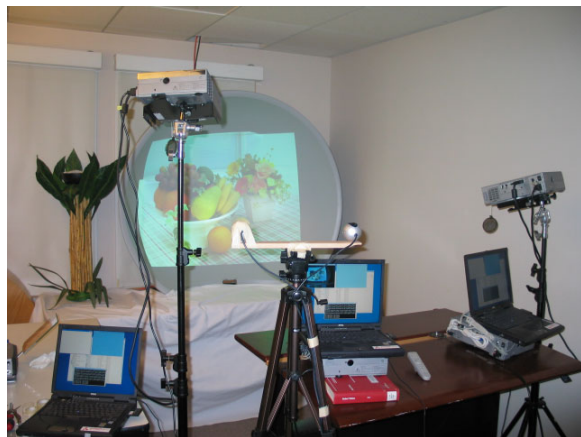
Figure 6: The setup of four casually installed projectors and stereo camera pair with a concave dome. The camera pair is not near the sweet spot.
