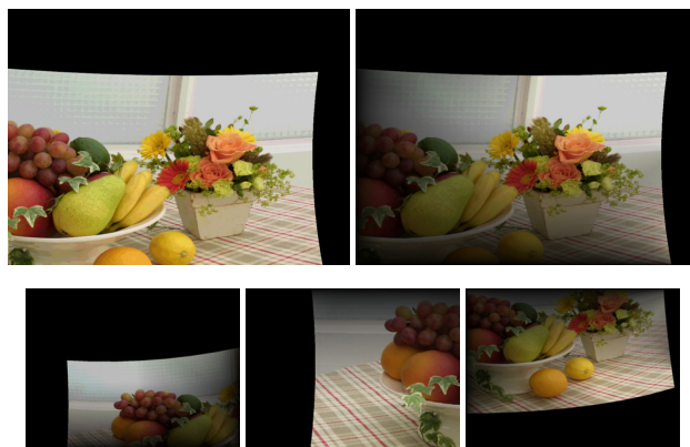
Figure 3: Top row: Image in top-right projector’s framebuffer, before and after attenuation with alpha map \Phi_i . Bottom row: Other three projectors with intensity correction. Note the outer black areas which are automatically generated after quadric transfer.
